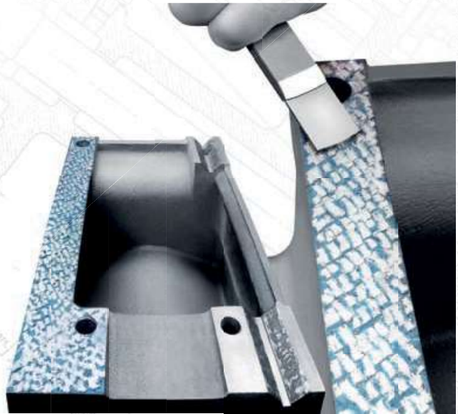
▲ Hand scraping of important parts – high precision during machining
